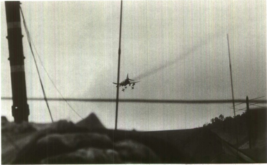
Marine F-4B Phantom delivers Snakeeye bombs on enemy trenches. Large tail fins retard the descent of the bombs. (Photo courtesy David D. Duncan)
